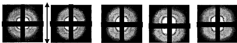
Fig. 7. Two-dimensional SAXS patterns from carbon black N330 dispersed in cross-linked SBR. From left to right: before stretching, stretched at \varepsilon=0.33 , \varepsilon=0.27 , \varepsilon=0.40 , \varepsilon=0.53 .
