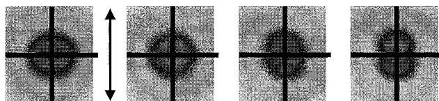
Fig. 13. Two-dimensional SAXS patterns from Aerosil R974 (hydrophobic) dispersed in uncross-linked EPR. From left to right: before stretching, stretched at \varepsilon=0.03 , \varepsilon=0.11 , \varepsilon=0.17 .
